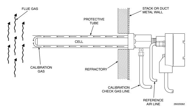
Figure 3-3. Proper Calibration Check Gas Flow Rate
